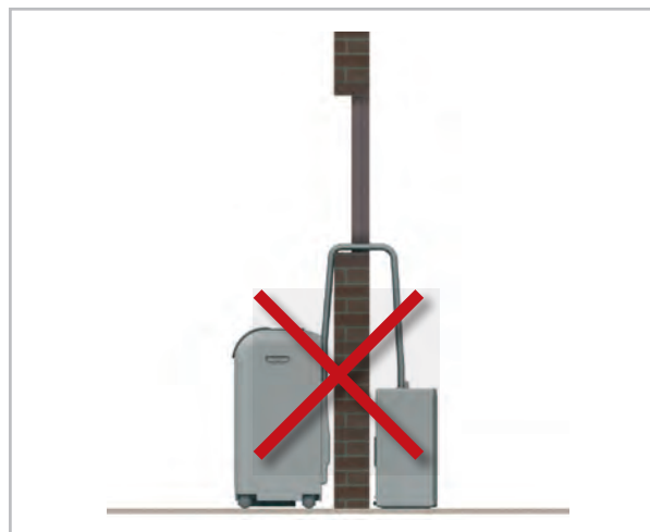
Fig. 6: Absence of minimum gap
